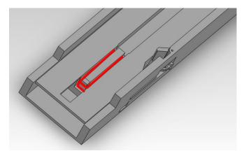
Install first the rubber band on the back side of the n°3 piece, because it's the more difficult to install
