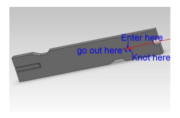
5) Install the first dentist rubber band on the bottom of the n°3 parts, next fixe it to part n°2 and do the same on the top:
