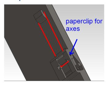
It's a difficult part to put the lock in the part n°4, Think about pass the rubber first around the lock and pass it in the whole in part n°4.
