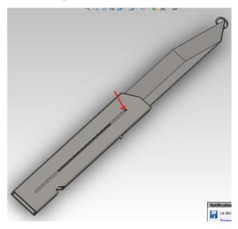
Put a paper clip on the blade whole and be sure that the paper clip block the blade but don't exceed the part n°4. The blade has to move smoothly!
